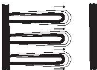
With U-bend tubes, there's room to expand, no contact or rubbing.
