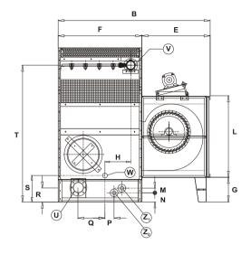
CT Cooling Tower with right hand side connection
