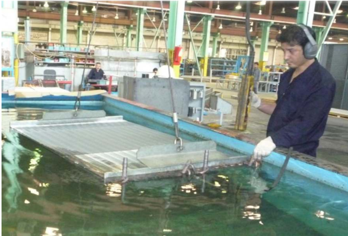
Pressure Test of Heat Exchangers
