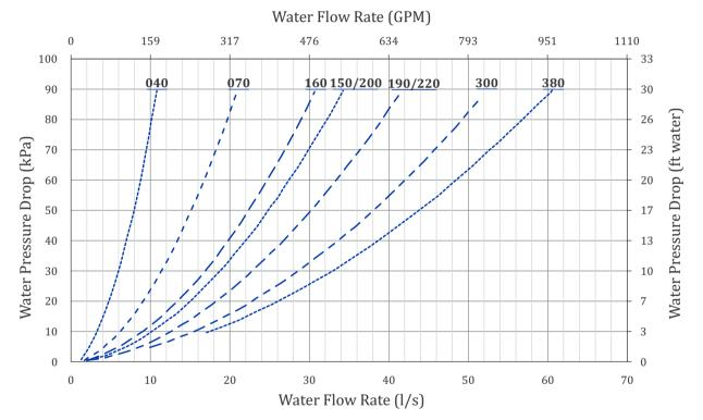
Cooler Pressure drop for different evaporator sizes
